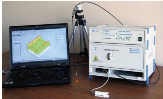
**Figure 1** Non-invasive multifunctional laser diagnostic system “LAKK-M”. It combines laser fluorescence diagnostics, pulse oximetry technique, laser Doppler flowmetry and tissue reflectance oximetry.
