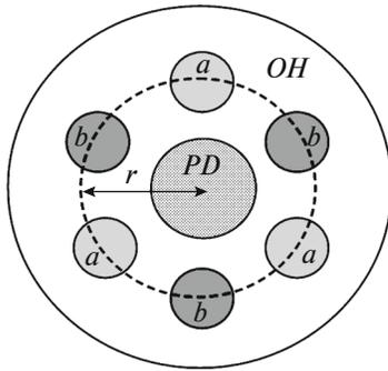
**Fig. 4.** The arrangement of the LED radiators (*a*, in the green spectral range of 560–580 nm and (*b*) in an IR range of 800–820 nm) and the photodetector *PD* in the optical head *OH* of the proposed device.
