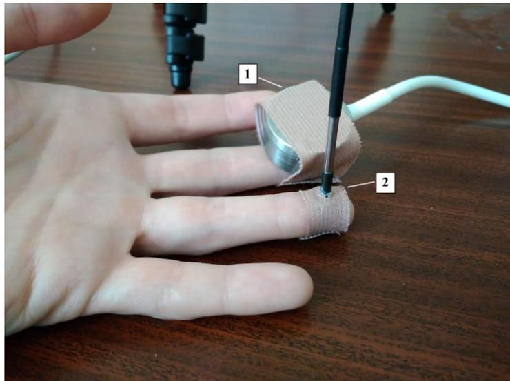
**Fig. 8.** Placement of the optical sensor of the developed device (1) and fiber probe of the l.d.f. instrument "LAKK-02" (2) on the subject's hand during the measurements.
