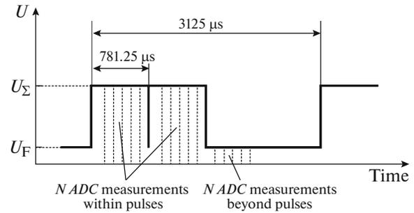
**Fig. 5.** The time diagram of the control pulses and the moments of signal digitization in the *ADC*.
