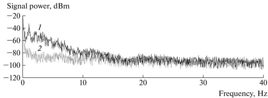
**Fig. 1.** The spectral density of the power of an amplitude-modulated signal that was recorded from the fingertip of a healthy volunteer in vivo (1) at rest and (2) at the moment of arterial blood-flow occlusion.
