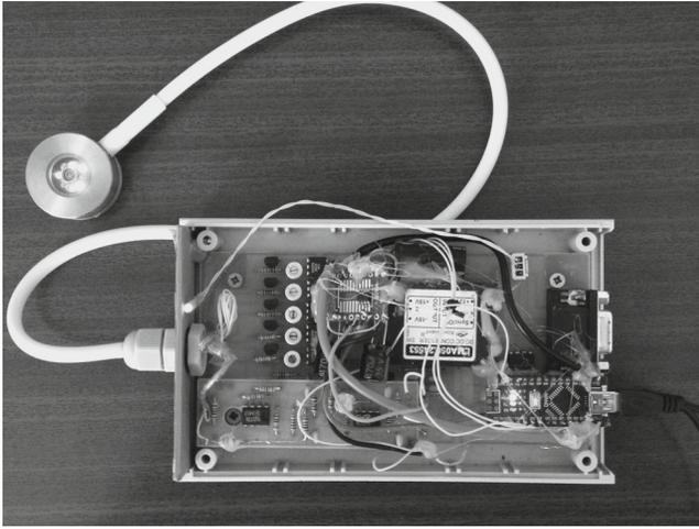
**Fig. 2.** The appearance of the developed device for measuring the skin blood flow.
